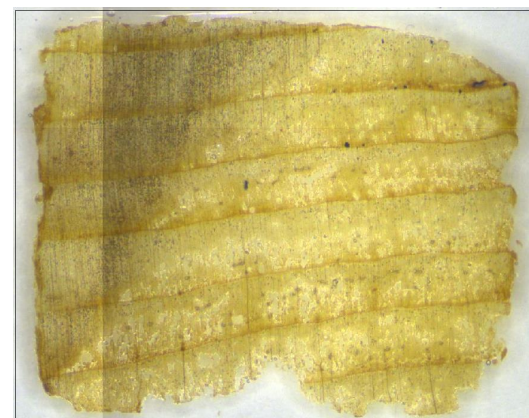
Embedded wood thin section ( \approx 200 \mu\text{m} )
